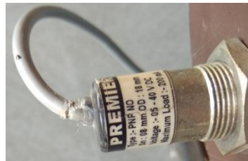
FIGURE A.5 : Proximity sensor for speed sensing
