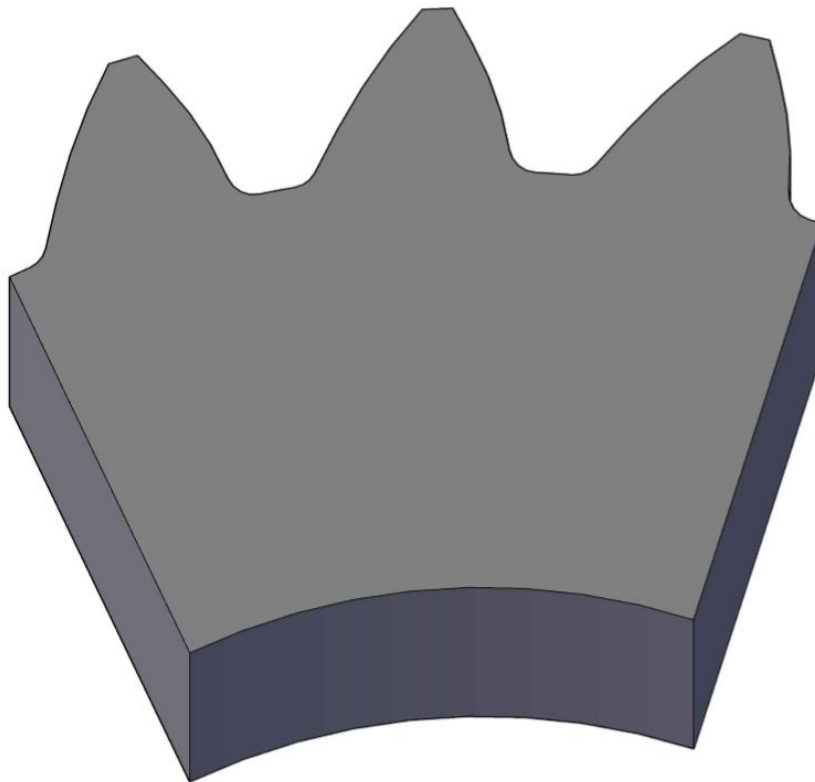
FIGURE 8.11: CAD model of segment of asymmetric involute spur gear ( \alpha_d=38^\circ , \alpha_c=20^\circ ) with normal fillet ( \rho_F=1.2 mm) at root of tooth
