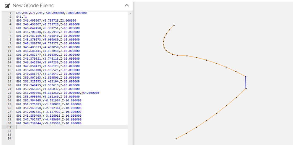
FIGURE 11.5: G code simulation for asymmetric gear with modified root profile
