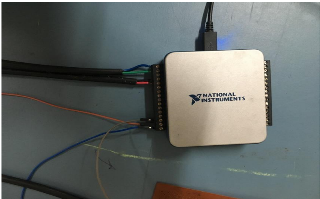
FIGURE: 6.4 National Instruments USB based Data acquisition Card 6001
