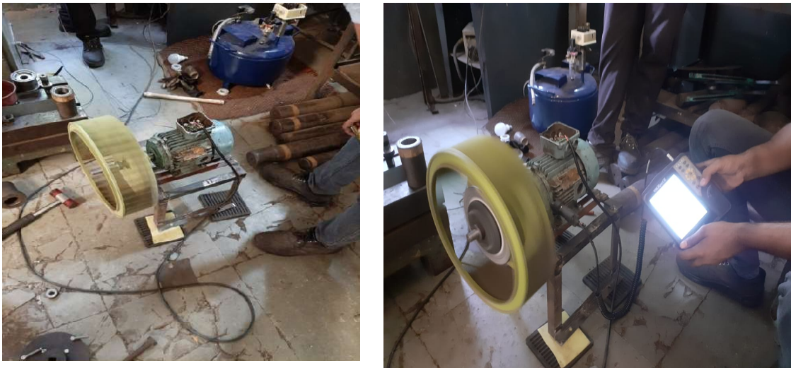
Figure 12: Experimental investigation of blower setup with DVA
