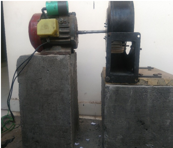
Figure 7: Blower setup without DVA.
