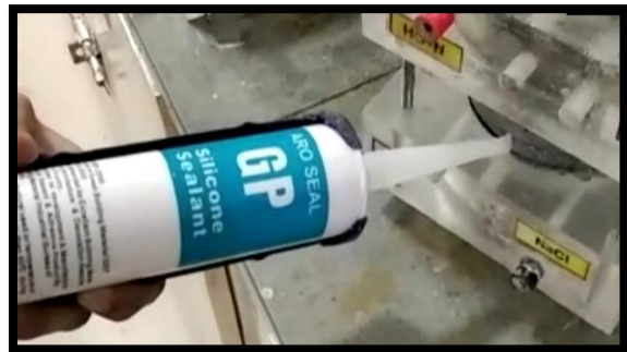
Fig.9 Casting and demolding of RCPT test mold Fig.10 Used silicon sealant to seal the gap between the concrete specimen and cell wall
