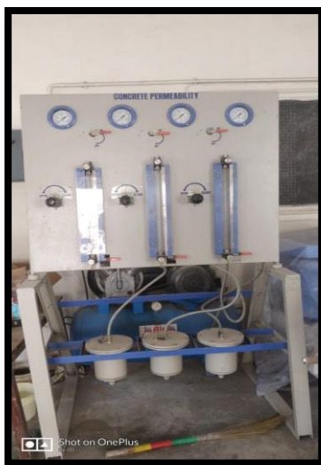
Fig.7 Water permeability test apparatus
