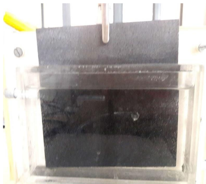
Fig. 4.7 Formation of bubbles on the surface of the electrode
