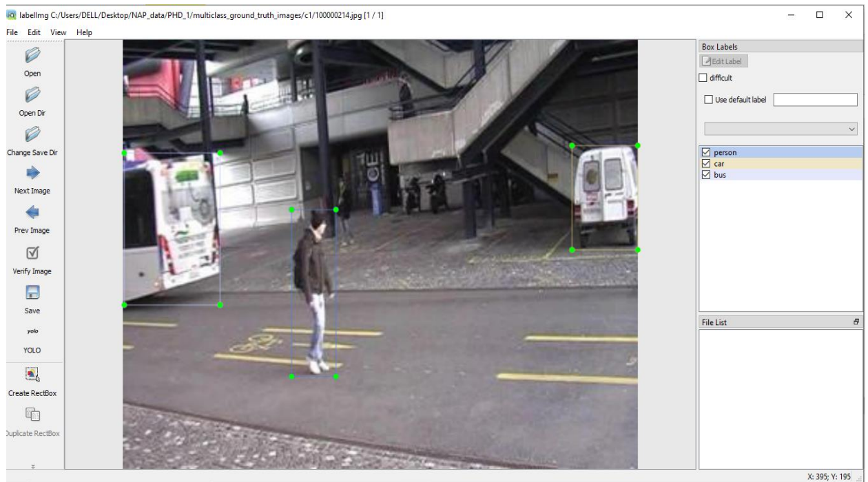
FIGURE 4.2 Sample annotated image in YOLOv7 format using labelImg tool
